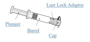
Hold the syringe by the barrel, not by the plunger.
